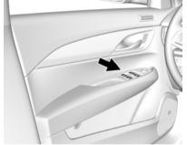
The power windows only operate with the ignition in ACC/ACCESSORY or ON/RUN/START, or when Retained Accessory Power (RAP) is active. See *Retained Accessory Power (RAP) on page 9-19*.
