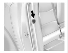
1. Remove the guide from its storage pocket on the side of the seat.
