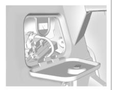
The rear compartment fuse block is behind a cover on the driver side of the rear compartment.
