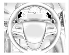
If equipped, the tap shift controls are on the back of the steering wheel.
