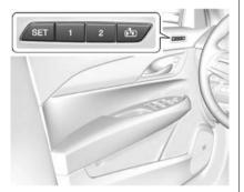
If equipped, the "1," "2," SET, and (Exit) buttons on the driver door are used to manually save and recall memory settings for the driver seat and outside mirrors.
