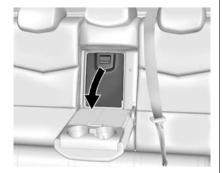
There is a rear seat pass-through door in the centre of the rear seatback. Fold down the centre armrest and pull the latch to open the door.
