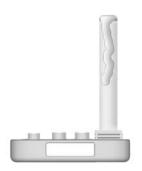
This key, inside the Remote Keyless Entry (RKE) transmitter, is used for the driver door and glove box.
