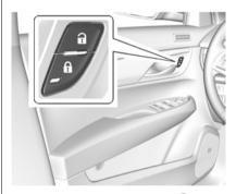
From the inside, press or or a. The indicator light in the switch will illuminate when activated. See Power Door Locks on page 2-11.
