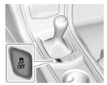
Manual Gearbox TCS/StabiliTrak Button Shown, Automatic Transmission TCS/StabiliTrak Button Similar
