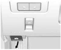
Pull the bonnet release handle inside the vehicle. It is on the lower left side of the instrument panel.
