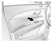
The power windows only operate with the ignition in ACC/ACCESSORY or ON/RUN/START, or when Retained Accessory Power (RAP) is active. See Retained Accessory Power (RAP) on page 9-19.
