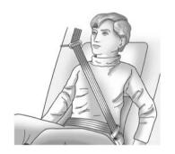
Buckle, position, and release the safety belt as described previously in this section. Make sure the shoulder portion of the belt is on the shoulder and not falling off of it. The belt should be close to, but not contacting, the neck. To remove and store the comfort guide, squeeze the belt edges together so that the safety belt can be removed from the guide. Store the guide in its storage pocket on the side of the seatback.
