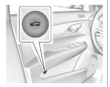
To open the boot, press from inside the vehicle or press from on the Remote Keyless Entry (RKE) transmitter, or push the touch pad on the rear of the boot above the number plate. See Remote Keyless Entry (RKE) System Operation on page 2-2 and Boot on page 2-12.
