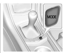
Manual Gearbox Mode Button Shown. Automatic Transmission Mode Button Similar
