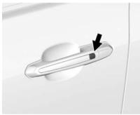
If equipped, use the Keyless Access system to lock and unlock the door. When the doors are locked and the Remote Keyless Entry (RKE) transmitter is within 1 m (3 ft) of the driver door handle, press the lock/ unlock button. When unlocking from the driver door, the first press unlocks that door; press again within five seconds to unlock all passenger doors. See Remote Keyless Entry (RKE) System Operation on page 2-2.
