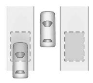
The SBZA sensor covers a zone of approximately one lane over from both sides of the vehicle, or 3.5 m (11 ft). The height of the zone is approximately between 0.5 m (1.5 ft) and 2 m (6 ft) off the
