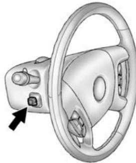
Push the control up or down to tilt the steering wheel up or down.
