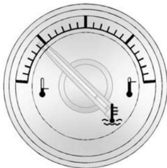
This gauge shows the engine coolant temperature.
