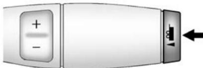
The vehicle has a Tow/Haul Mode. The Tow/Haul Mode adjusts the transmission shift pattern to reduce shift cycling, providing increased performance, vehicle control, and transmission cooling when driving down steep hills and mountain gradients, towing, or hauling heavy loads.
