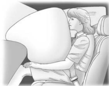
The front outboard passenger frontal airbag is in the instrument panel on the passenger side.
