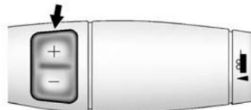
The DSC switch is located on the shift lever.
