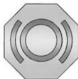
The brake master cylinder reservoir is filled with DOT 3 brake fluid. See *Engine Compartment Overview on page 10-5* for the location of the reservoir.
