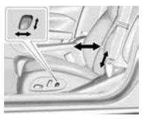
If equipped, to increase or decrease the lumbar support, press and hold the control forward or rearward or up and down.
