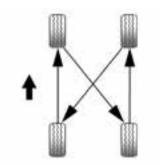
Use this rotation pattern when rotating tyres of the same size installed on all four wheel positions.
