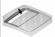
Dirt and debris may collect on the sunroof seal or in the track. This could cause an issue with sunroof operation or noise. It could also plug the water drainage system. Periodically open the sunroof and remove any obstacles or loose debris. Wipe the sunroof seal and roof sealing area using a clean cloth, mild soap, and water. Do not remove grease from the sunroof. If water is seen dripping into the water drainage system, this is normal.
