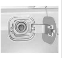
To open the fuel filler flap, push and release the rearward centre edge of the flap. If equipped, the fuel door is locked when the vehicle doors are locked. Press and on the RKE transmitter to unlock.
