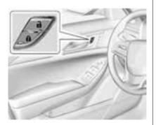
From inside, press **a** or **a**. The indicator light in the switch will illuminate when activated. See *Power Door Locks on page 2-11*.
