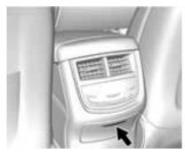
If equipped, press the top of the door to open the storage area on the rear of the centre console. If equipped, there is a power outlet inside.
