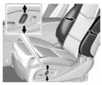
If equipped, to adjust the bolster support, press and hold the recliner control up and down.
