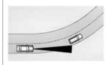
When following a vehicle and entering a bend, ACC may not detect the vehicle ahead and accelerate to the set speed. When this happens the vehicle ahead symbol will not appear.
