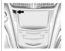
(Hazard Warning Indicators): Press and hold this button for one second to make the front and rear indicator lamps flash on and off. Release the button for at least one second and press again to turn the flashers off.
