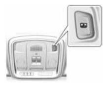
If equipped with a rear window sunshade, the switch is on the overhead console. The sunshade only operates with the ignition in ON/RUN/START.
