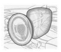
The driver frontal airbag is in the centre of the steering wheel.
