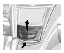
Touch the bottom of the climate control system panel until the door automatically starts to open. The storage area may contain a USB port, SD card reader, and auxiliary jack. See the infotainment manual.
