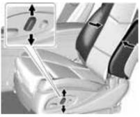
If equipped, to increase or decrease the seatback bolster support, press and hold the recliner control up and down.
