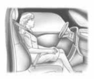
If a person of adult size is sitting in the front outboard passenger seat, but the off indicator is lit, it could be because that person is not sitting properly in the seat. Use the following steps to allow the system to detect that person and enable the front outboard passenger frontal airbag and knee airbag:
