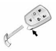
Press the button to remove the key. The key can be used for all locks.
