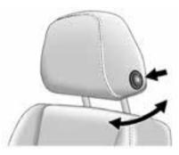
To adjust the head restraint forward and rearward, press the button located on the side facing the head restraint and move it forward or rearward until the desired locking position is reached. Try to move the head restraint after the button is released to make sure that it is locked in place.
