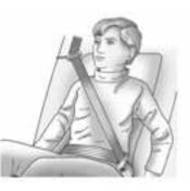
4. Buckle, position, and release the safety belt as described previously in this section. Make sure the shoulder portion of the belt is on the shoulder and not falling off of it. The belt should be close to, but not contacting, the neck. To remove and store the comfort guide, squeeze the belt edges together so that the safety belt can be removed from the guide. Store the guide in its storage pocket on the side of the seatback.
