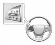
(S) (On/Off): Press to turn the system on and off. A white indicator appears in the instrument cluster when cruise is turned on.
