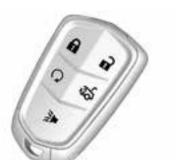
**(Lock):** Press to lock all doors. The indicator lamp indicators may flash and/or the horn may sound to indicate locking. See "Remote Lock, Unlock, Start" under *Vehicle Personalisation on page 5-47*.
