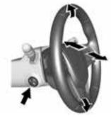
If equipped, the control is on the left side of the steering column.
