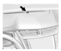
The solar sensor, on top of the instrument panel near the windscreen, monitors the solar heat.
