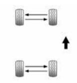
Use this rotation pattern if the vehicle has different size tyres on the front and rear and they are non-directional.
