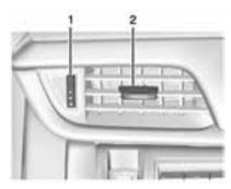
Move the slider knobs (2) to change the direction of the airflow.
