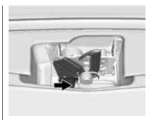
2. Go to the front of the vehicle to find the secondary bonnet release handle. The handle is under the front edge of the bonnet near the centre. Push the handle to the right and at the same time raise the bonnet.
