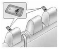
Top-tether fastening eyes are marked with log for a child seat.
