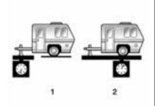
The trailer tongue (1) should weigh 10 to 15 percent of the total loaded trailer weight (2).
