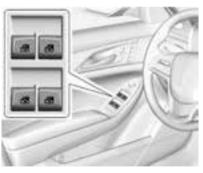
The driver power window switches control all the windows. The passenger switch only controls that window.
