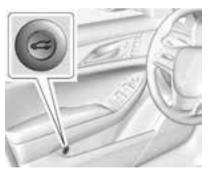
To open the boot, press in the driver door, press twice quickly on the Remote Keyless Entry (RKE) transmitter, or press the touch pad on the rear of the vehicle after unlocking all doors.
