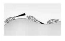
Do not use ACC when driving on steep hills or when towing a trailer. ACC will not detect a vehicle in the lane while driving on steep hills. The driver will often need to take over acceleration and braking on steep hills, especially when towing a trailer. If the brakes are applied, the ACC disengages.
