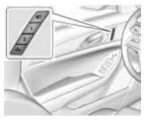
The SET, "1," "2," and D (Exit) buttons on the driver door are used to manually save and recall memory settings for the driver seat, outside mirrors, and power tilt and telescoping steering column (if equipped).
