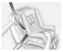
4. To tighten the belt, push down on the child restraint, pull the shoulder portion of the belt to tighten the lap portion of the belt, and feed the shoulder belt back into the retractor. When installing a forward-facing child restraint, it may be helpful to use your knee to push down on the child restraint as you tighten the belt.
