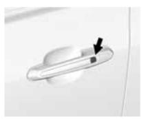
Use the Keyless Access system to lock and unlock the door. When the doors are locked and the Remote Keyless Entry (RKE) transmitter is within 1 m (3 ft) of the driver door handle, press the lock/unlock button. When unlocking from the driver door, the first press unlocks that door; press again within five seconds to unlock all passenger doors. See *Remote Keyless Entry (RKE) System Operation on page 2-2.*
