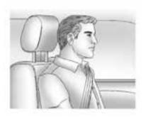
Adjust the head restraint so that the top of the restraint is at the same height as the top of the occupant's head. This position reduces the chance of a neck injury in a crash.
