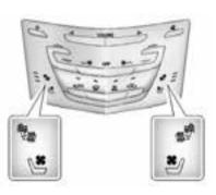
If equipped, the buttons are near the climate controls on the centre stack. To operate, the ignition must be in ON/RUN/START.
