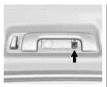
Press the button next to each rear passenger reading lamp.
