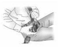
If the webbing locks in the catch plate before it reaches the buckle, tilt the catch plate flat to unlock.
