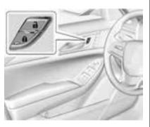
**(Lock):** Press to lock the doors. The indicator light in the switch will illuminate when activated.
