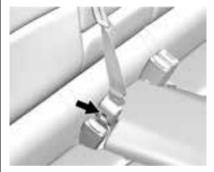
1. Disconnect the rear safety belt mini-latch using a key in the slot on the mini-buckle, and let the belt retract.
