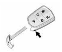
1. Press the button on the side of the transmitter near the bottom and pull the key out.
