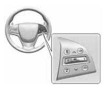
$<sup>\</sup>wedge$  or  $\vee$ : Press to move up or down in a list.
