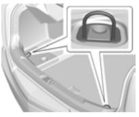
The cargo tie-downs can be used to secure small loads inside the boot.
