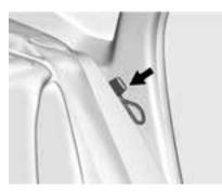
1. Remove the guide from its storage pocket on the side of the seat.
