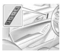
The SET, "1," "2," and D (Exit) buttons on the driver door are used to manually save and recall memory settings for the driver seat, outside mirrors, and power tilt and telescoping steering column (if equipped).
