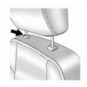
To lower the head restraint, press the button, located on the top of the seat backrest, and push the head restraint down. Try to move the head restraint after the button is released to make sure that it is locked in place.
