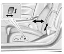
If equipped, to adjust the lumbar support, press and hold the control forward or rearward or up and down. See Lumbar Adjustment on page 3-4.
