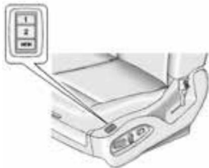
The “1,” “2,” and MEM buttons on the outboard side of the driver seat are used to manually save and recall the positions of the driver seat, outside mirrors, and adjustable throttle and brake pedal positions.
