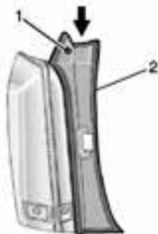
2. Remove the push pin (1) on the tail lamp cover (2).
