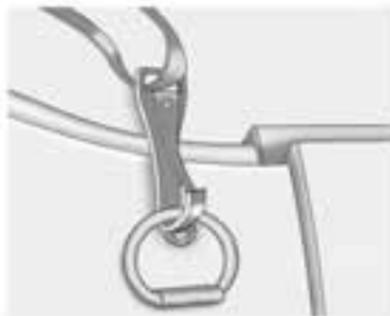
5. Attach the strap to the cargo tie-down in the rear of the vehicle.
