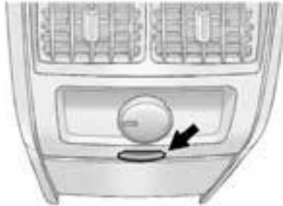
Press the button to open the storage area on the rear of the centre console. If equipped with Rear Seat Entertainment (RSE), the audio/video jacks, USB port and SD card reader may be inside. See the infotainment manual.
