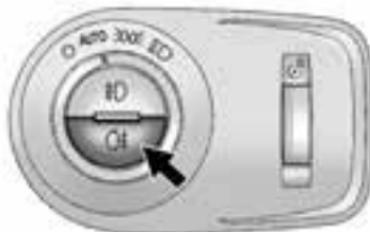
The rear fog lamp button is on the exterior lamp control, on the outboard side of the steering wheel.
