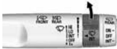
**INT (Rainsense Wipe Sensitivity Control):** Move the windscreen wiper lever to INT. Turn the
