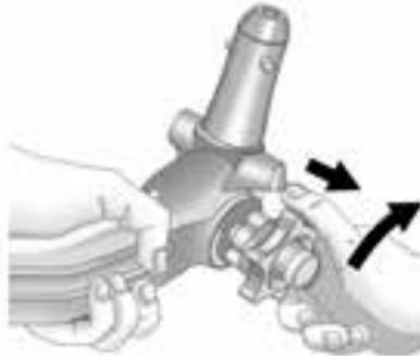
3. If the hitch is not ready to be installed, the tension must be set by pulling the knob out and turning it clockwise as far as it will go.
