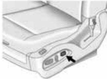
Press and hold the front or rear of the control to increase or decrease lumbar support. Release the control when the seatback reaches the desired level of lumbar support.
