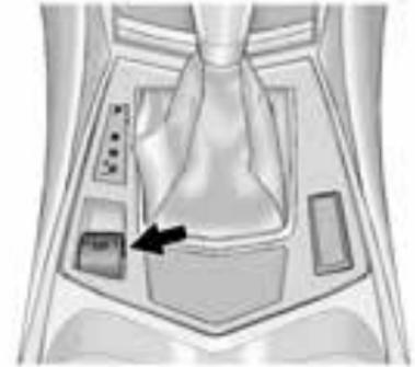
The Electric Parking Brake (EPB) switch is on the centre console. The EPB can always be activated, even if the ignition is off. To prevent draining the battery, avoid repeated cycles of the EPB when the engine is not running.
