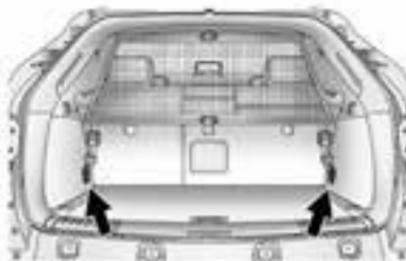
5. Mount the cargo net to the cargo tie-downs on the lower side panels.
