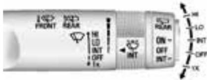
With the ignition in ACC/ACCESSORY or ON/RUN/START, move the windscreen wiper stalk to select the wiper speed.
