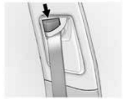
Move the height adjuster up to the desired position by pushing up on the height adjuster.
