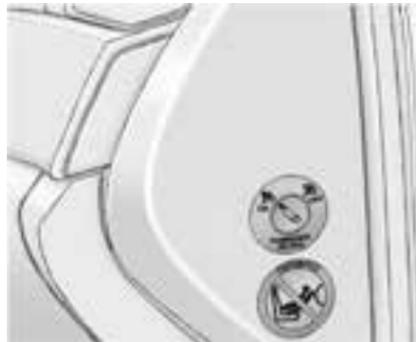
This switch should only be turned to the off position if the person in the front outboard passenger position belongs to a category indicated in this section:
