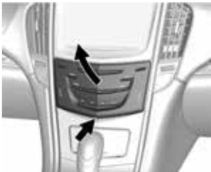
If equipped with storage behind the climate control system, touch and hold the chrome bar at the bottom of the climate control system panel to open. There is a USB port inside. See “USB Port” in the infotainment manual.
