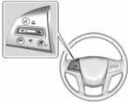
**CC** : Press to turn the system on and off. A white indicator appears in the instrument cluster when cruise is turned on.
