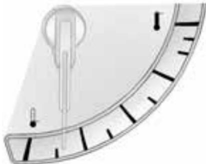
This gauge measures the temperature of the vehicle's engine. If the needle moves into the shaded area while driving under normal operating conditions, the engine is too hot. Pull off the road, stop the vehicle, and turn off the engine as soon as possible.
