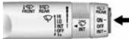
**ON:** Press the upper portion of the button for continuous rear window wipes.
