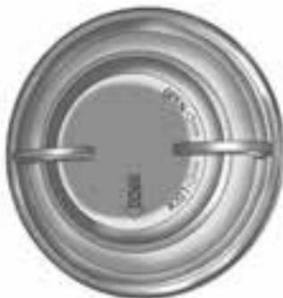
2. From the back side of the headlamp assembly, remove the bottom cap to replace the main beam headlamp bulb.
