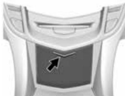
A storage area is located in front of the gear lever. Push upward on the top of the door and release; the door automatically opens.
