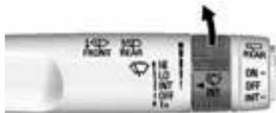
**INT:** Move the windscreen wiper lever to INT. Turn the
