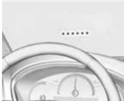
If ACC is engaged, driver action may be required when ACC cannot apply sufficient braking because of approaching a vehicle too rapidly.
