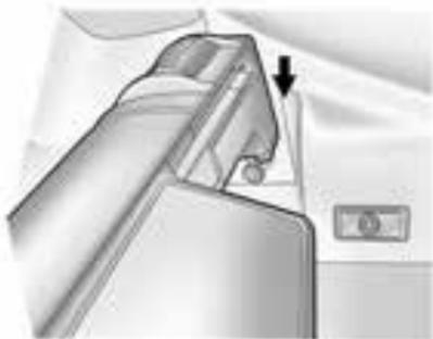
2. Align the cartridge over the pins on the trim panels of the vehicle.
