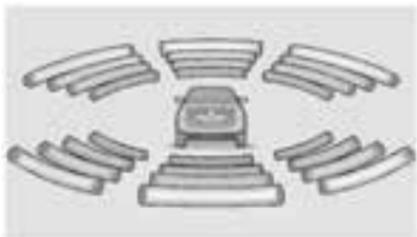
The instrument cluster may have a parking assist display with bars that show “distance to object” and object location information for the Parking Assist system. As the object gets closer, more bars light up and the bars change colour from yellow to amber to red.
