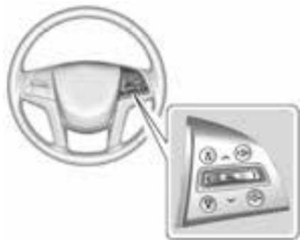
**^ or v** : Press the five-way control to move up or down in a list.
