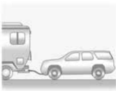
To tow the vehicle from the front with all four wheels on the ground:
