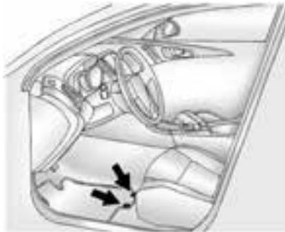
1. Pull up on the rear of the floor mat to unlock each retainer and remove.
