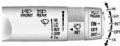
With the ignition in ACC/ACCESSORY or ON/RUN/START, move the windscreen wiper lever to select the wiper speed.
