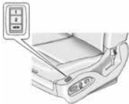
The "1," "2," and MEM buttons on the outboard side of the driver seat are used to manually save and recall the positions of the driver seat, outside mirrors, and adjustable throttle and brake pedal positions (if equipped).
