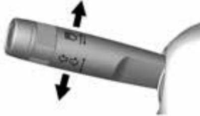
Move the lever all the way up or down to signal a turn.
