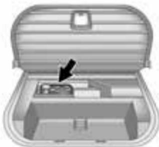
This vehicle may have a tyre sealant and compressor kit in place of a jack or spare tyre. It is located
