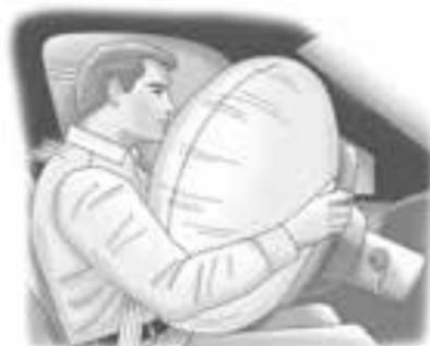
The driver frontal airbag is in the centre of the steering wheel.
