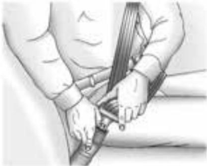
To unlatch the belt, just push the button on the buckle.
