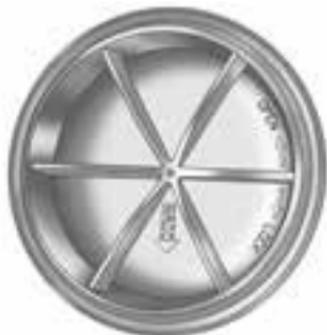
1. From the back side of the headlamp assembly, remove the top cap to replace the dipped beam headlamp/DRL bulb.
