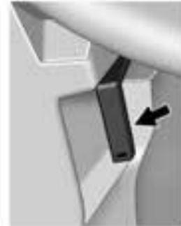
1. Pull the release handle with the above symbol on it. It is located below the instrument panel to the left of the steering wheel.
