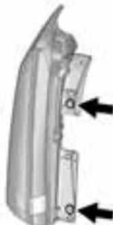
4. Remove the two screws from the taillamp assembly.
