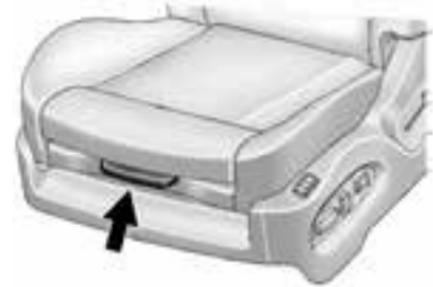
Adjust the manual leg extension by pulling up on the lever, and then pulling or pushing on the support to lengthen or shorten it. Release the lever to lock it in place.
