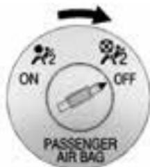
To turn off the front outboard passenger frontal airbag, insert any key or a coin into the switch, push in, and move the switch to the off position.
