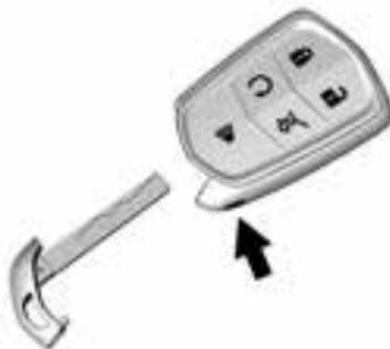
1. Press the button on the side of the transmitter near the bottom and pull the key out.
