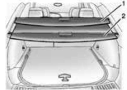
The shade can be set in two positions. It can be set in a halfway open (1) position for loading objects
