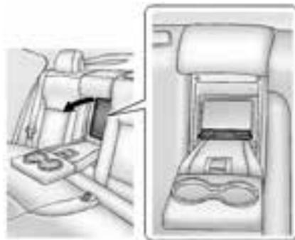
There is a rear seat pass-through door in the centre of the rear seatback. Fold down the centre armrest and push down on the latch to open the door.
