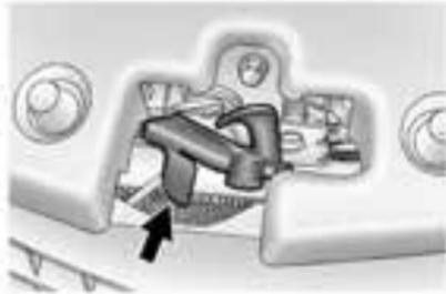
2. Move the secondary bonnet release lever up to release the striker. The lever is located near the middle of the bonnet.
