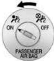
To turn the front outboard passenger frontal airbag on again, insert any key or a coin into the switch, push in, and move the switch to the on position.
