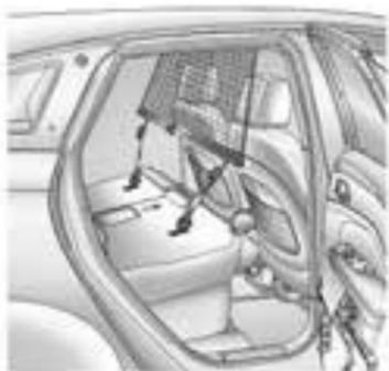
3. Mount the cargo net to the rear seat tethers on the back of the folded down rear seats and pull on the straps to tighten the net.
