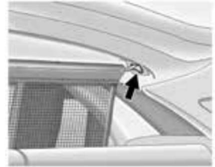
1. Insert the top corners of the cargo net into the large openings in the headlining and secure by sliding them into the small openings.
