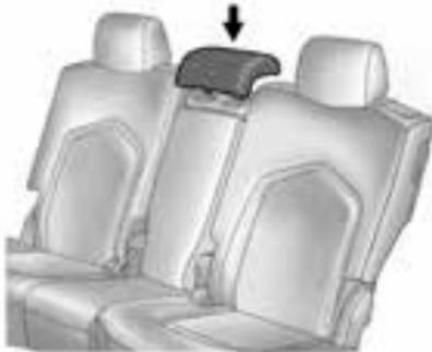
The vehicle's rear seat has an adjustable headrest in the centre seating position that can be adjusted the same way as the outboard head restraints.
